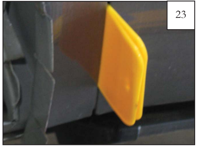
To prevent paint damage, insert body filler spreader or plastic spacer between fender and door. This will keep the fender from hitting the door edge while pounding back sheet metal in the next few steps.
