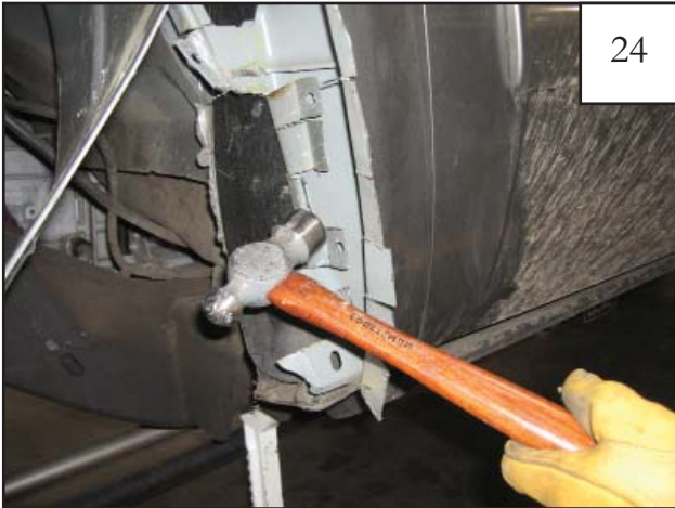
Bend inner support over and use a hammer to flatten against wall inside fender.
