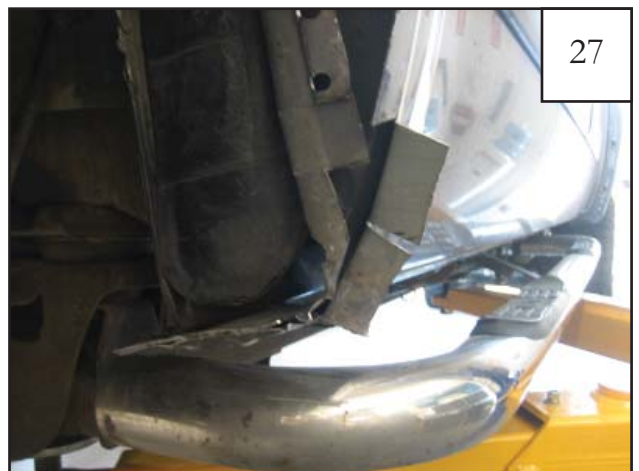
Bend remaining metal back even with other tabs. Note: Remove any additional overlap.
