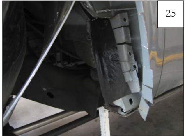
Inner flange flush against wheel well wall.
