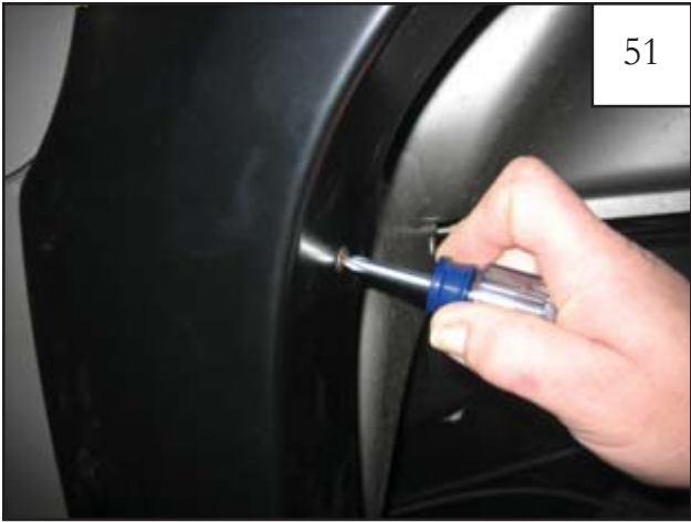
Reposition flare on fender. Start a supplied serrated flange screw through each of the remaining holes and into each "S" clip installed in step 50.
