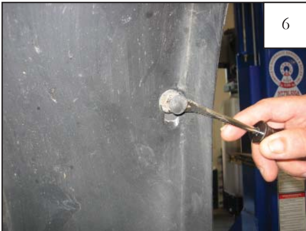
Using a pry tool, remove plastic factory fastener from wheel well liner.
