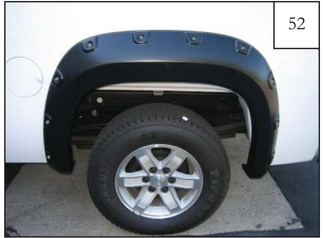
Completed rear flare installation.
