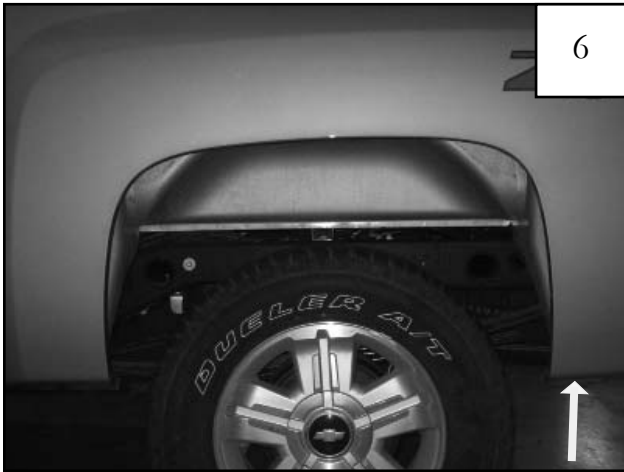
Remove one factory bolt with a 1/2" wrench.
