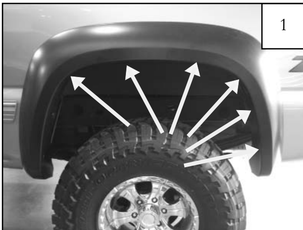
Remove six factory fasteners with a pry tool.
