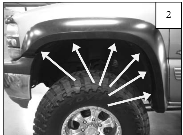
Install six tuflocks using a #2 stubby screwdriver.
