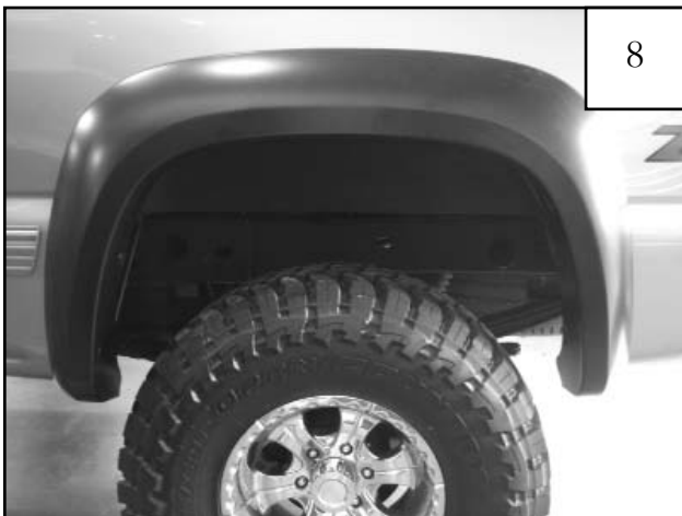
Completed rear flare installation.
