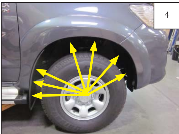
Remove seven factory screws from the fender lip. Save screws for reinstallation. Remove flare by pulling part away from side of vehicle.
