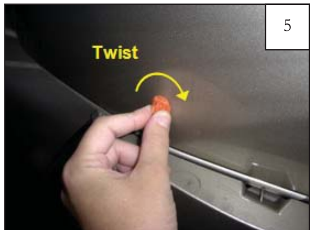
Using a clockwise twisting motion, remove six factory plastic clips from fender. See step 7.
