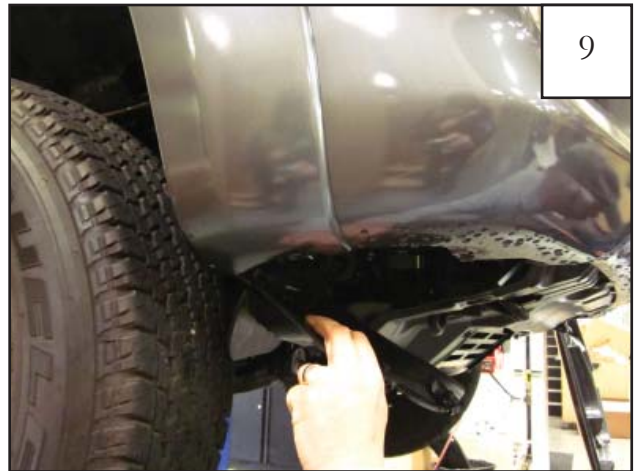
Pull down bumper cover and splash shield.
