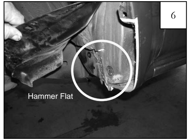
Using a hammer, flatten the fire wall weld seam as shown. Removing the wheel and tire is recommended for work clearance.
