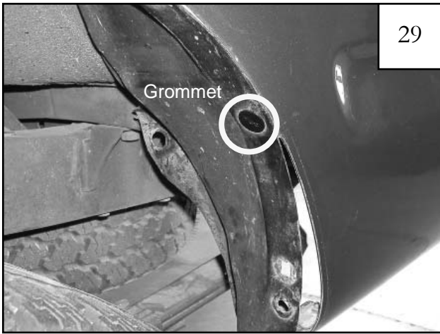
29 Install kit-supplied Grommet (GR1-0001) into the REAR splash shield as shown, refastening the shield to the body.
