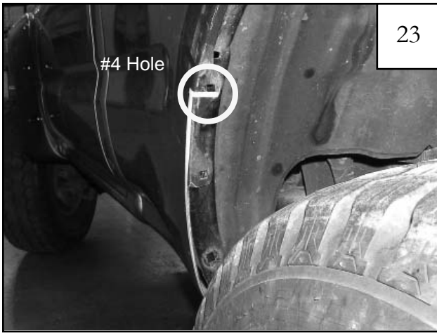
FRONT - Using the 4th hole up from the bottom as a guide, make a tape line along lower edge of hole horizontally.
