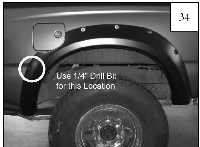
34 Remove fasteners and flare. For hole specified in photo, drill hole with a 1/4" drill bit, ensuring to keep the drill level and perpendicular to fender surface.
