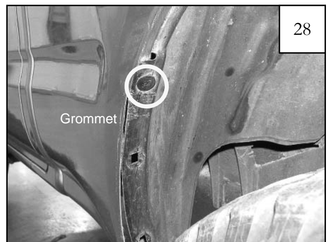
Install kit-supplied Grommet (GR1-0001) into the FRONT splash shield as shown, refastening the shield to the body.
