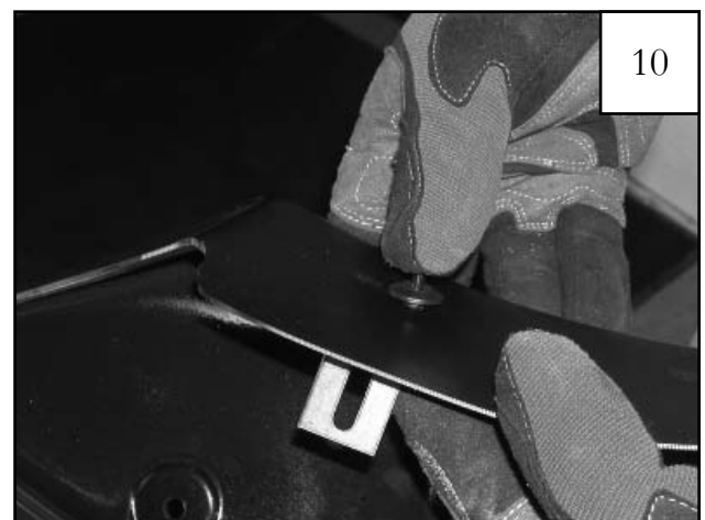
Install the kit-supplied Bracket (MB1-0008) on the flare with a Retainer (RV1-P001). The Bracket should angle down from the inner flare surface.
