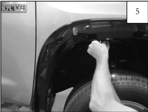
Place flare on fender, aligning holes with clips on the bracket. Start two supplied 20mm Hex Screws (SW1-0036) through two holes on the top of the flare and into clips.
