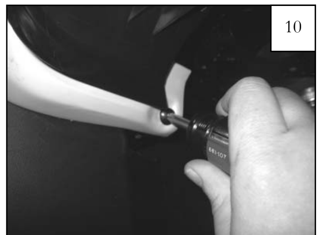
Start a supplied Serrated-Flange screw through lower rear hole in flare and into "S" Clip installed in Step 9. Tighten all screws.
