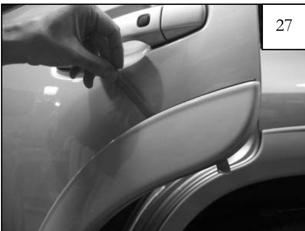
While holding the Door Piece in place, pull upper tape liner tab.
