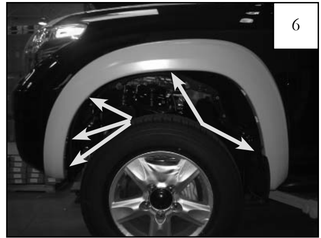
Reposition Front Flare on Fender. Hand start five supplied Hex Screws through flare and into hole locations shown (three in wheel well, one at front underside of bumper, and one through the "U" Clip installed on bracket in Step 11). Do not tighten.
