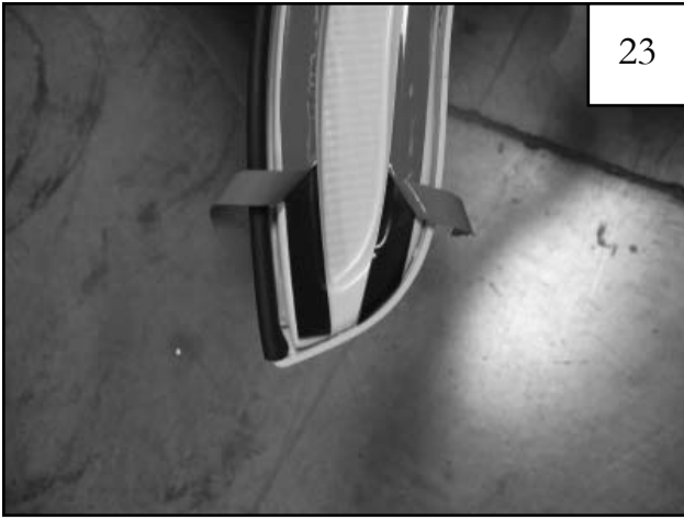
Fold red liner of Door Piece tape toward the outside of the part. (Make sure the tabs are folded toward the outside of the part.)
