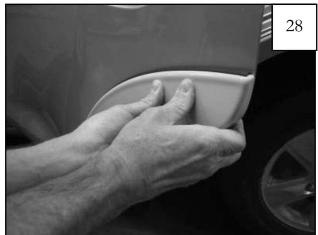
Press the part into place. Brace fingers on inside of door and use thumbs to press firmly against part and repeat along full length of part at upper tape liner location. Tape reaches maximum adhesive bond after 24 hours of contact.
