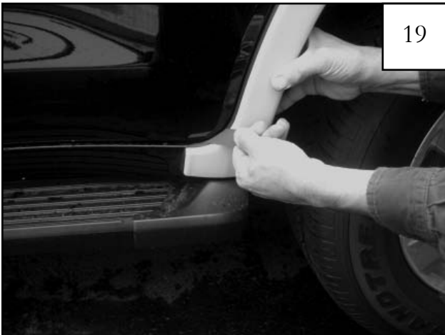
While holding bottom front edge of flare in place, pull the tape tab. Press part into place, applying 30 PSI for a minimum of 15 seconds for proper bond. Once tape adheres, parts should not be adjusted in this area.
