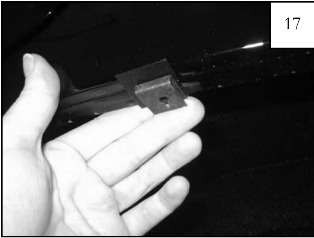
Position four "S" Clips onto fender lip over Black Tabs.
