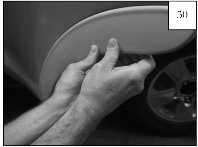
Brace fingers on inside of door and use thumbs to press firmly against part and repeat along full length of part at lower tape liner location. Tape reaches maximum adhesive bond after 24 hours of contact.
