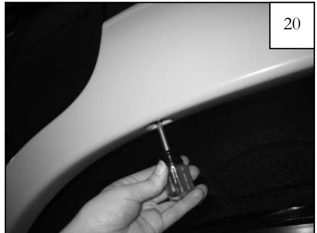
Start four supplied Serrated-Flange Screws through forward holes in flare and into "S" Clips installed in Step 17, starting with topmost hole and working your way down. Once last screw is started, tighten all screws.
