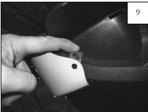
Slide an Clip/Black Tab combination (CL1-0005/MT1-0002) onto bumper lip, aligning with hole located at front underside of flare.
