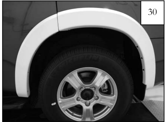
Once all screws have been started, apply pressure towards vehicle at each fastening point as you tighten all screws.
