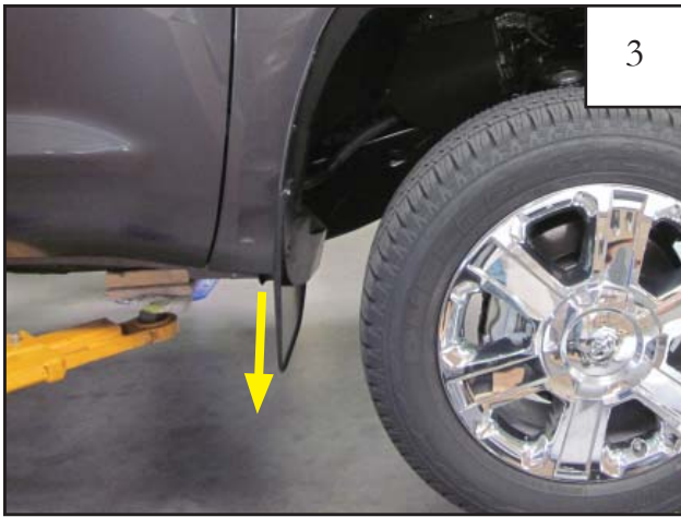
3 Remove factory push retainer from underside of factory mud guard. Remove mud guard from vehicle.
