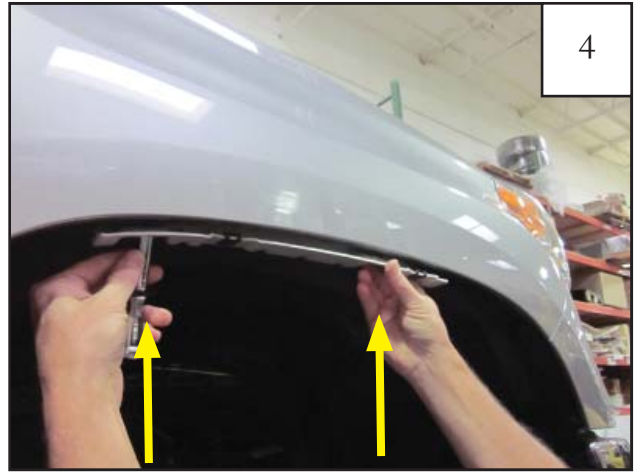
4 Using two supplied 20mm Hex Screws (SW1-0036), attach bracket to factory holes with a 10mm socket.
