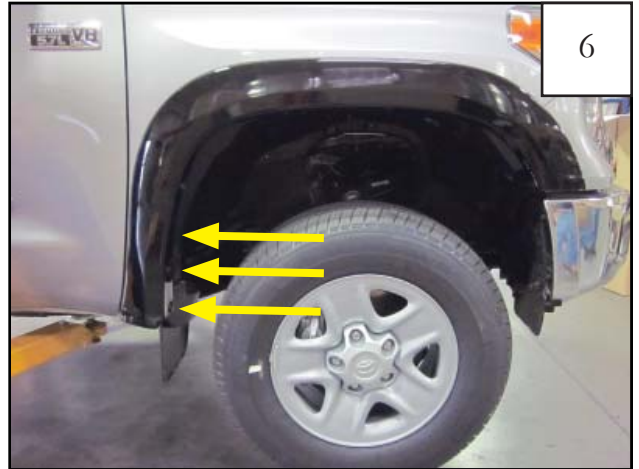
6 Start three supplied 20mm Hex Screws (SW1-0036) through three rear holes in flare and into factory holes in rear of wheel well.
