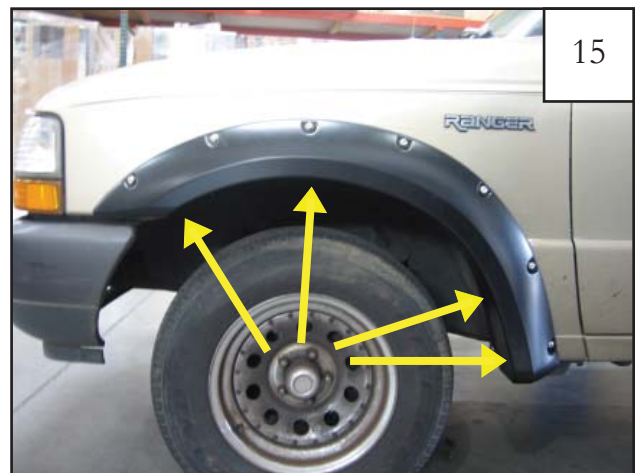
Ensuring proper flare placement, tighten all screws.
