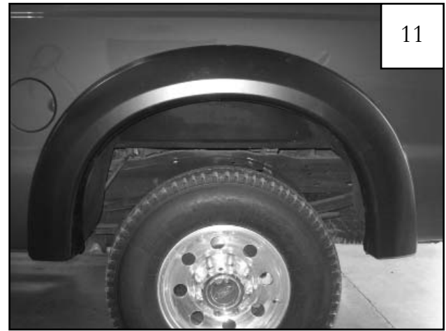
Completed rear flare installation.
