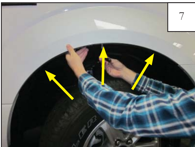
Using a 7/32" socket wrench, reinstall the factory screws through the inner piece.
