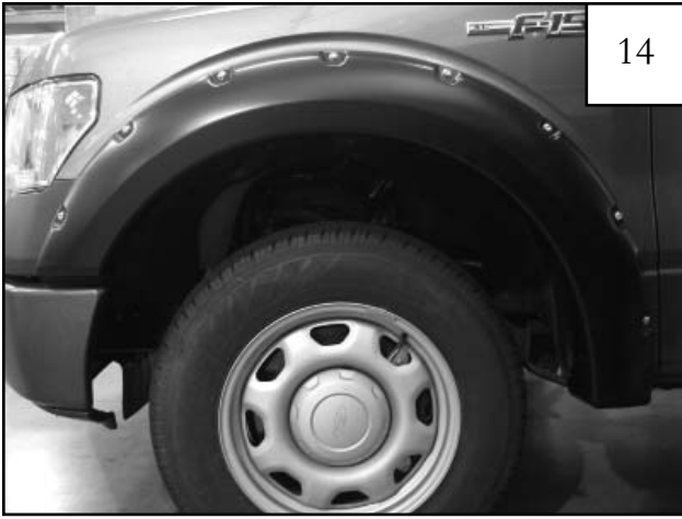
Completed front flare installation.
