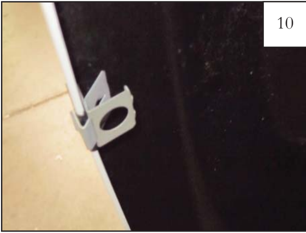
Center clips on the tabs installed in Step 8 and push onto the bumper cover.
