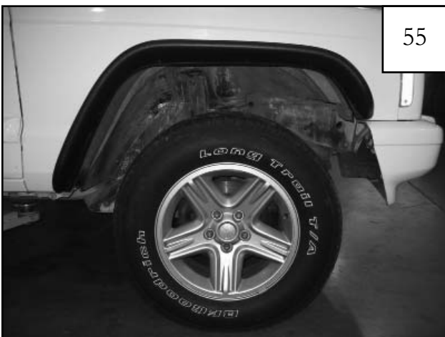
Completed front passenger's side flare installation.
