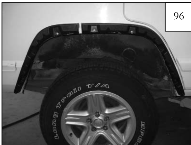
Inner pieces installed.
