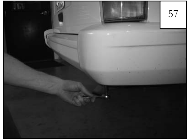
(For 97-01 Model Years Only) Remove the factory bumper rear fastener using a 10mm socket & wrench.
