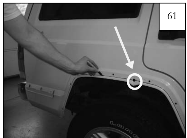
Use a grease pencil or marker to mark a line on the style line closest to the wheel well of the fender for trimming. Ensure that marked line does not go past the first style line. All factory mounting holes should remain intact after trimming. (For 97-01 Model Years Only) The larger factory hole indicated in picture may be cut in half.
