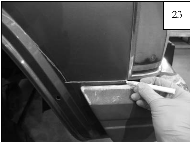
(For 84-96 Model Years Only) Use a grease pencil or marker to make a horizontal line extending from bottom of front marker light to profile line made in step 22.
