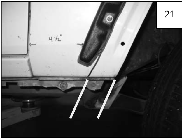
At end of inner pieces extend trimming line so that it is parallel with the wheel well opening instead of following inner piece curvature.
