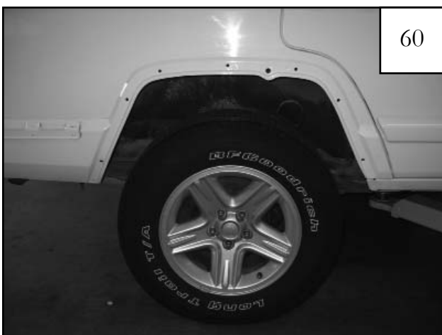
With the factory flares removed, thoroughly clean the exposed metal fender with a damp cloth and dry. (For 97-01 Model Years Only) Pop out two factory panel retainers to remove splash shield.
