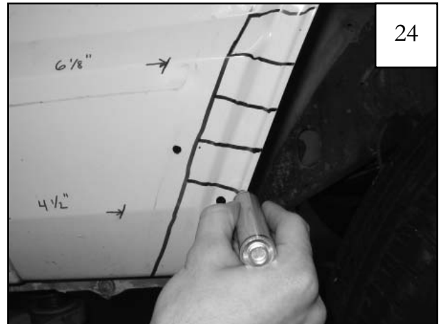
Remove inner pieces. Mark horizontal lines 1.5" apart starting on lower rear style line of sheet metal and ending on upper horizontal style line in sheet metal.
