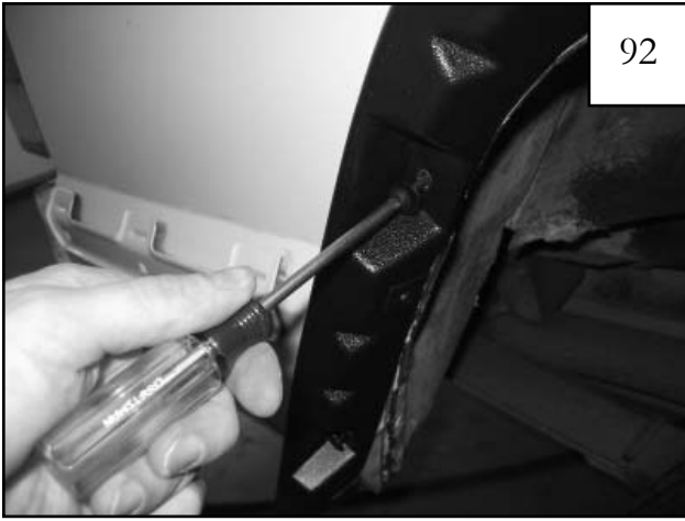
Position inner pieces on fender and tighten screw, washer, spacer combo using a #2 Phillips bit. Do not overtighten.
