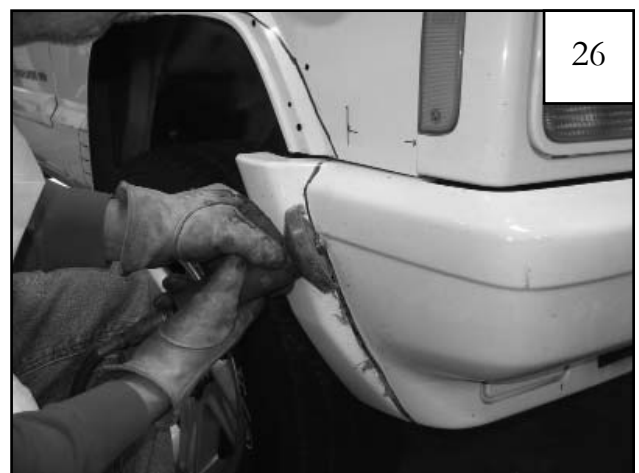
(For 97-01 Model Years Only) Use a cut off saw to cut front bumper along marked line.
