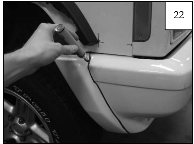
(For 97-01 Model Years Only) Use a grease pencil or marker to make a line on the factory front bumper for trimming.
