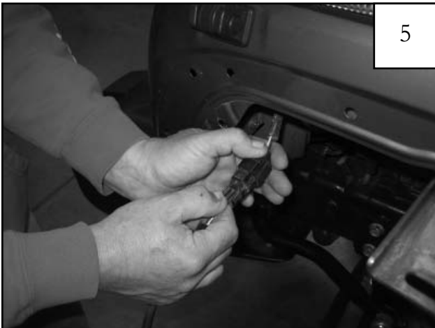
Once flare is free of fender, disconnect light connector. This will allow the flare to come away from fender completely. Save connector for reinstallation.
