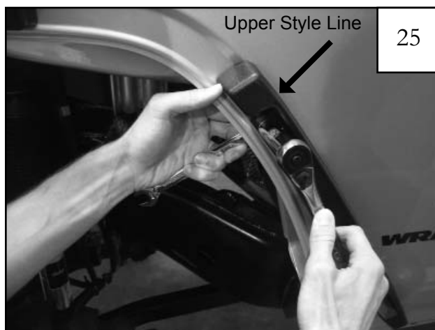
Step 3 Using a 1/2" socket wrench and a 1/2" wrench, tighten all bolts until inner piece is snug against fender. Do not overtighten: see step 21. Inner piece should rest along upper style line of sheet metal radius and not below it: see step 22.
