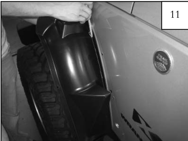
Using sheet metal as a guide, mark the rear portion of the splash shield with a grease pencil in preparation for trimming. The splash shield should be flush with the sheet metal after being trimmed. NOTE: If trimmed too little, flare won't fit; if trimmed to much, shield won't stay behind flare.
