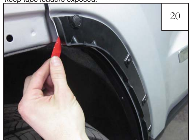
20 Remove red tape liner from inner piece.
