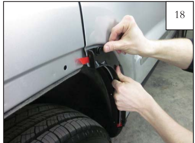
18 Hold Inner Door Piece against vehicle aligning upper hole with factory hole in sheet metal and the remaining three holes with grommets installed in Step 15. Install (1) provided Push Retainer (RV1-0014) into top hole to secure Inner Door Piece to vehicle. Note: Be sure to keep tape leaders exposed.
