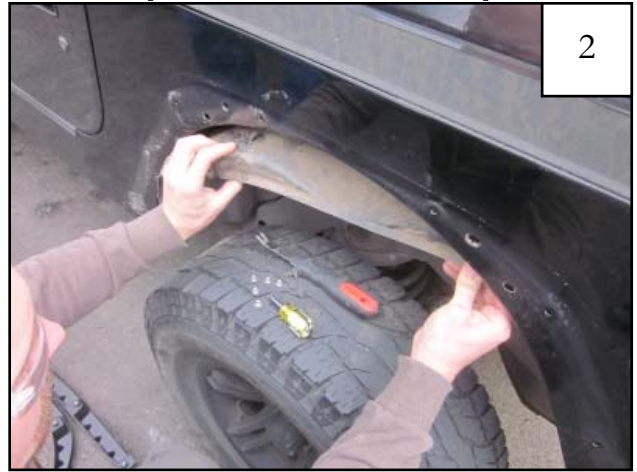
2 Using a pry bar or claw hammer, remove the christmas tree fasteners then remove/loosen the rear wheel well skirting. Save fasteners for reinstallation.
