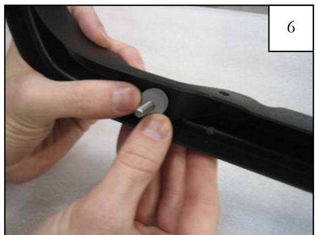
6 Push the rubber spacer and M5-8 machine screw together until they are both tight against the inner piece. Spacer has been lightened in picture for visibility.
