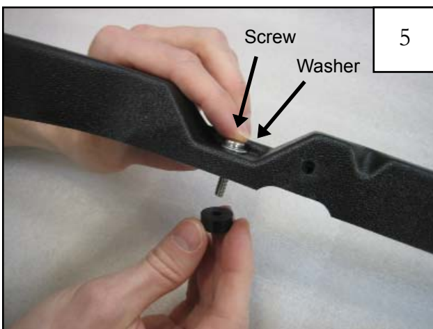
5 Put an M5-8 machine screw (SW1-0053) and washer (WA1-0003) through the top holes of the inner pieces and secure with a 1/4" rubber spacer (SP1-0011) on the underside of the inner piece.
