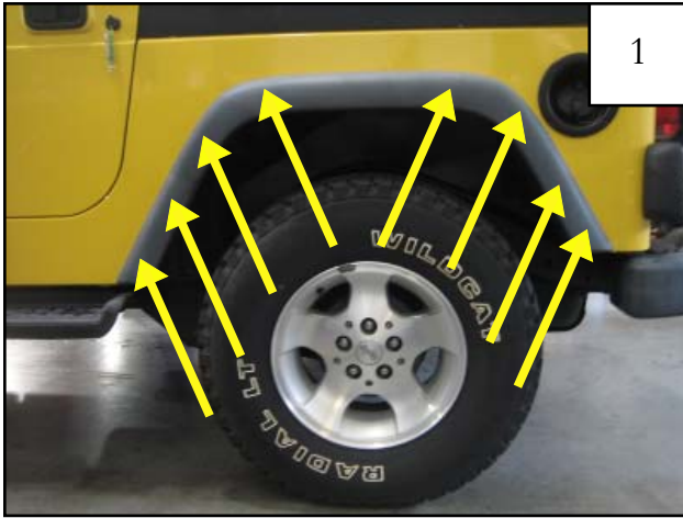
1 Remove the factory installed fender flare screws with a 5/16" socket wrench. (8 locations)
