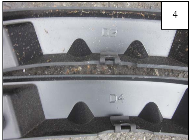
4 Locate the new flat flare rear inner pieces. The driver side rear inner pieces are marked D3 and D4. The passenger side rear inner pieces are marked P3 and P4.
