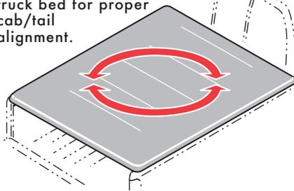
Carefully refold the tonno without shifting its position on the truck bed.
