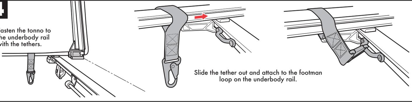
Slide the tether out and attach to the footman loop on the underbody rail.
