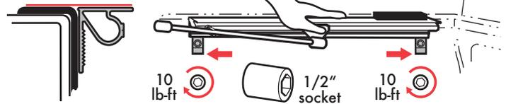
**2** Unfold the tonno fully and adjust position over the truck bed for proper cab/tail alignment.
