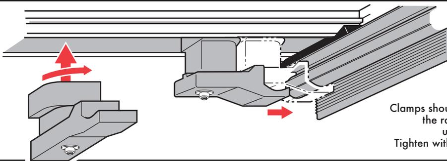
Clamps should be fully secured under the radius section of the underbody rail.
