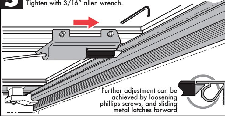
Further adjustment can be achieved by loosening phillips screws, and sliding metal latches forward
