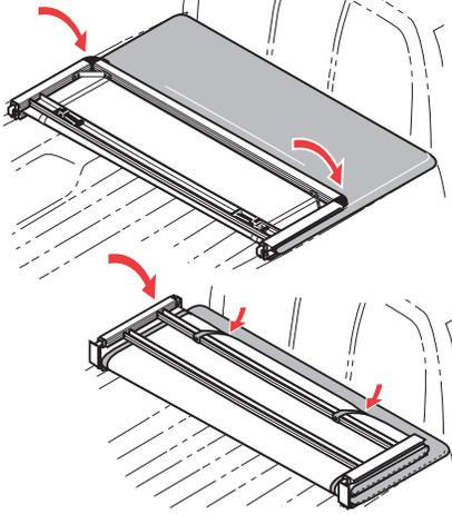
**IMPORTANT:** Before folding the second section of the tonno, rear clamps must be stowed into the rear bow to prevent damage to fabric.
