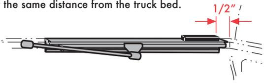
Align the top of the underbody rail flush with the top of the truck bed and secure the clamps as shown.
