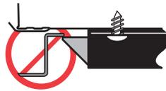
...hand-loosen latch screws and slide the latch toward the side rail. Retighten screws by hand.
