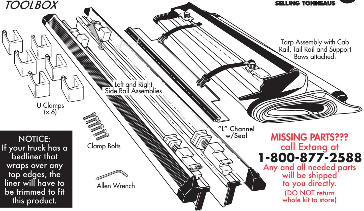
Tarp Assembly with Cab Rail, Tail Rail and Support Bows attached.
