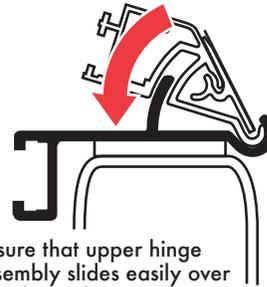
Make sure that upper hinge rail assembly slides easily over ridge on lower hinge rail.
