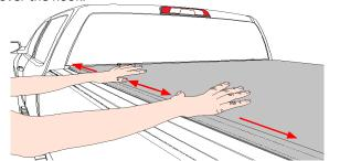
Next, run your hands down both sides of the cover. This will prevent wind from lifting the cover and causing possible damage.
