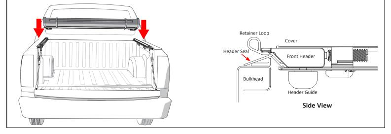
Slide right and left header guides into the locked position. A clicking sound will indicate a secure attachment. Your tonneau cover has been successfully installed.
