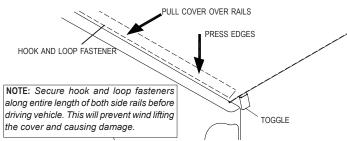
STEP 8: To release cover, Trigger pull rear release toggle. Start rolling cover toward cab making sure both sides of cover roll evenly. For best results leave unrolled portion of cover attached to the hook and loop fasteners while
