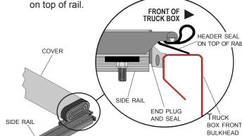
STEP 5: Tighten bolts but do not over tighten. Header must
