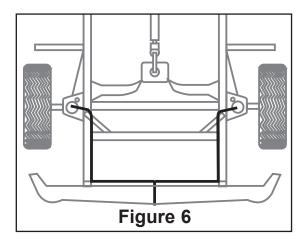
Tee air line installation recommended unless weight in vehicle varies from one side to the other and unequal pressures are needed to level the load. Dual air lines are used in this case.
