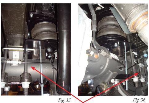
If the hard brake line is resting on the lower bracket carriage bolts on either side, push or pull the brake line out of the way.
