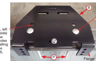
For models with sway bars, right (passenger side) only, use these holes for installing Carriage Bolts (B).
